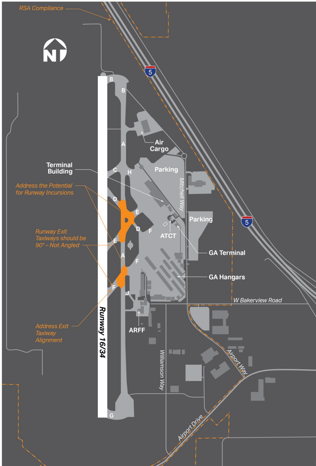
Figure 5-5: Taxiway Design Issues
